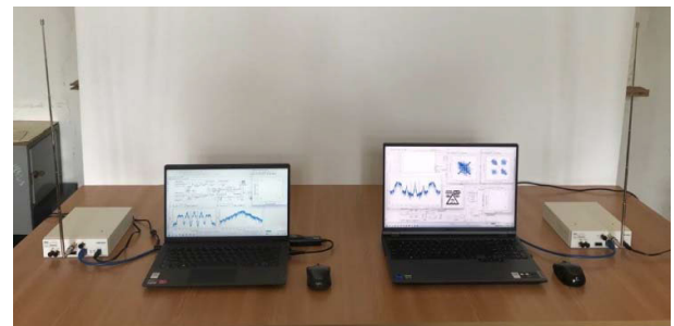
FIGURE 23. Experimental setup including two N210 USRPs configured as transmitter (left) and as receiver (right).
