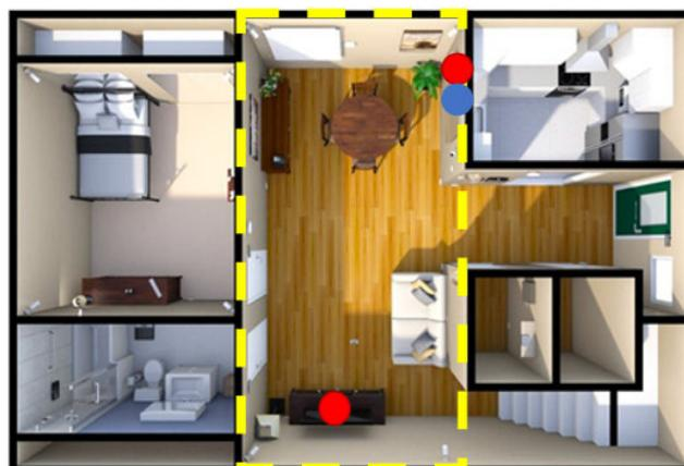
**FIGURE 1.** HomeLab layout at KITE Research Institute. The yellow box represents the areas in the field of view of the cameras, the red dots represent the locations of the RGB cameras and the blue dot represents the depth camera.
