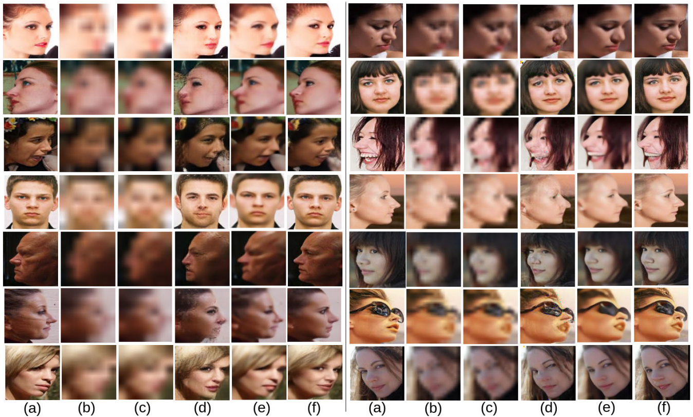
FIGURE 12. Qualitative SR comparison on the AFLW2000 dataset. Left part: (a) HR ( 128 \times 128 ), b) LR ( 8 \times 8 ), c) bicubic interpolation, d) ExtremeSR [69], e) MGBPv2 [76], and f) ours for the upsampling rate of \times 16 . Right part: a) HR ( 128 \times 128 ), b) LR ( 16 \times 16 ), c) bicubic interpolation, d) ProgFSR [32], e) SPARNet [77] and f) ours for the upsampling rate of \times 8 . Please zoom in to have a better detailed view of the images.
