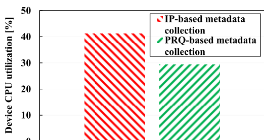
FIGURE 7. Comparison of IP-based and PRQ-based average device CPU utilization monitoring result.
