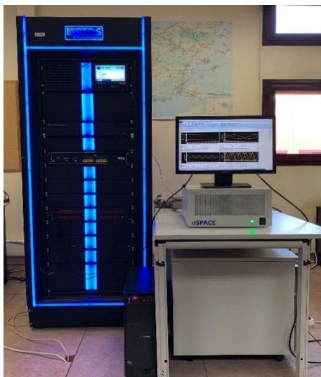
FIGURE 25. Hardware in the Loop experimental set-up.
