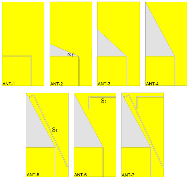
FIGURE 2. Schematic geometry of various antennas involved in the design evolution process. The yellow-colored parts were considered to be copper in the numerical models.
