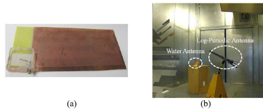
FIGURE 22. (a) Prototype of the F-Shaped wideband hybrid water monopole antenna developed in [57], (b) RC set-up for antenna efficiency measurement. (Reproduced from [57] under a Creative Commons Attribution 4.0 International License (CC BY 4.0)).
