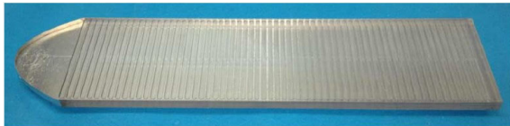
FIGURE 33. Prototype of the fabricated dynamic water grating leaky-wave antenna utilized in the developed antenna in [30]. (Reproduced from [30] with permission. Copyright ©2014 IEEE).
