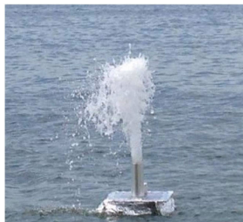
FIGURE 16. Photograph of the dynamic-type sea-water monopole antenna operated in real sea-side environment. (Reproduced from [25] with permission. Copyright ©2015 IEEE).
