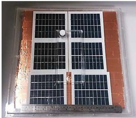
FIGURE 6. Prototype of the water dielectric patch antenna integrated with solar cells. (Reproduced from [23] under a Creative Commons Attribution 4.0 International License (CC BY 4.0)).
