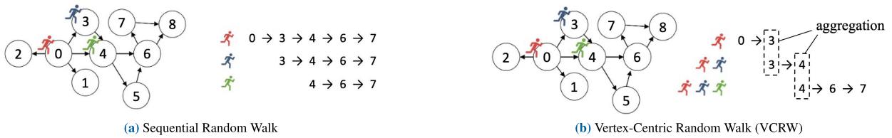
FIGURE 5. Assuming that there are three random walks from vertex 0, 3, and 4 that have the same path 4 \rightarrow 6 \rightarrow 7 , sequential random walks need to obtain neighbor vertices every time as shown in Fig. 5(a). On the other hand, VCRW can reduce the total number of operations to obtain neighbor vertices by aggregating three random walks at vertex 3 and vertex 4 as shown in Fig. 5(b).
