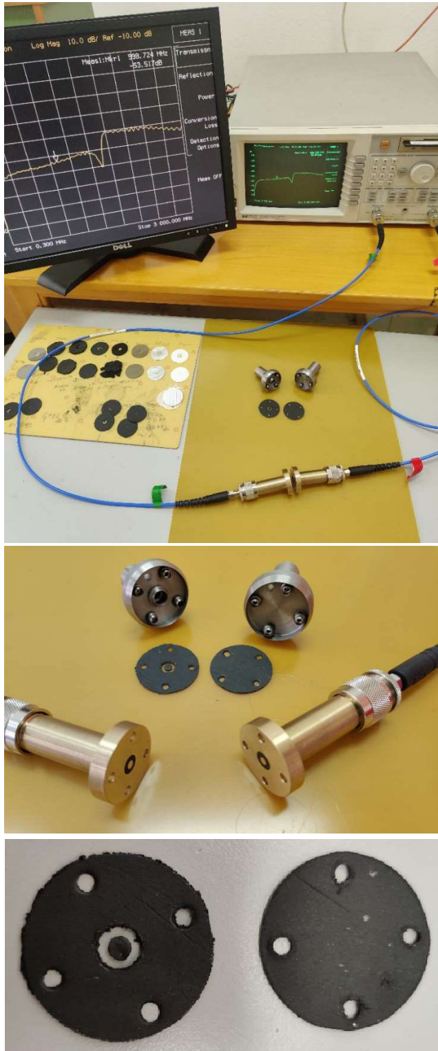
FIGURE 6. Top: SE monitoring equipment, middle: monitoring devices, bottom: close-up of OTB samples prepared for shielding effectiveness tests.
