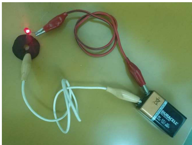
FIGURE 5. Photo demonstrating the low electric resistivity of biochar sample OTB3-AB20. The LED light turns on when a 5 V DC electric circuit supporting a red LED is in contact with the sample.
