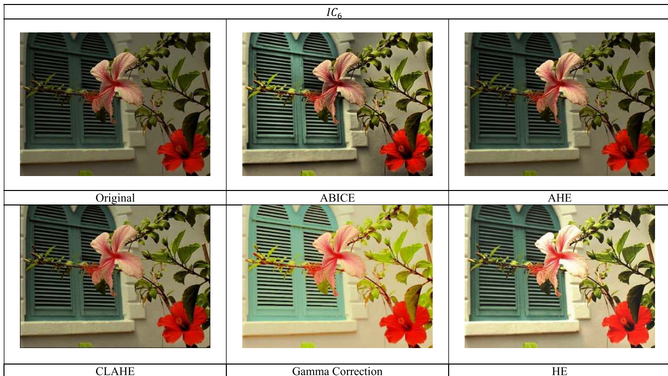
FIGURE 18. Contrast enhancement results of the color image IC_6 for ABICE, AHE, CLAHE, Gamma Correction, and HE methods.
