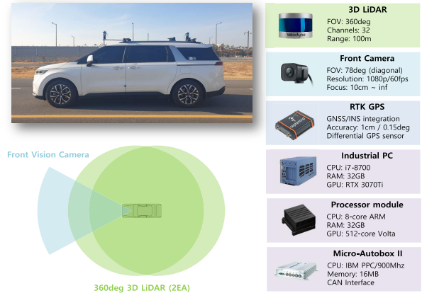
FIGURE 2. Hardware configuration of the autonomous test vehicle.
