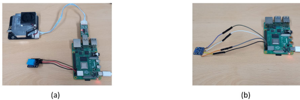
FIGURE 10. IoT devices with sensors; (a) nCube device with dust and humidity sensors, (b) IoTivity device with temperature sensor.
