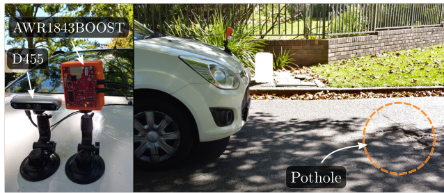
FIGURE 5. Bonnet-mounted experimental configuration of the D455 and AWR1843BOOST sensors. The remainder of the PDCL system was positioned inside the vehicle. The location of a pothole of interest has been highlighted in front of the vehicle.
