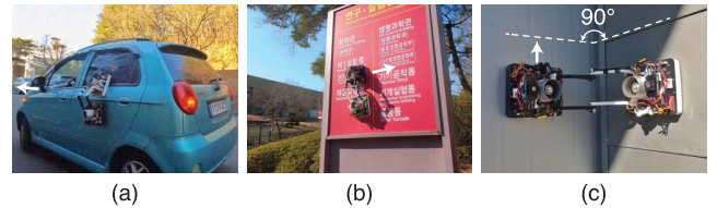
FIGURE 17. Attachment of proposed robot system on (a) accelerating car, (b) flat wall, and (c) 90°-angled wall.
