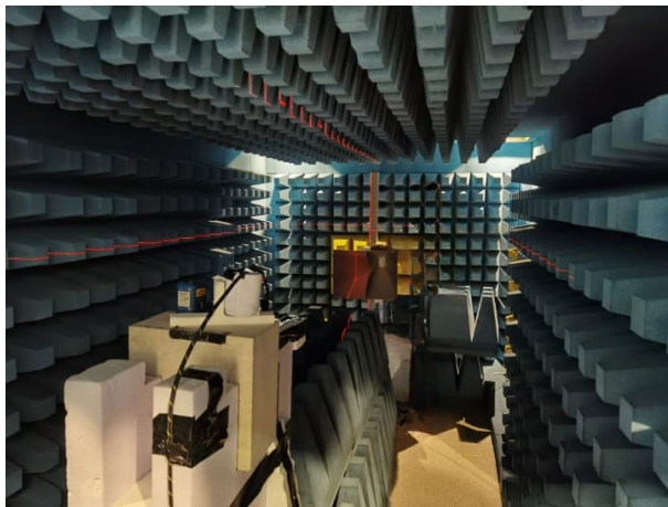
FIGURE 2. Photograph of the actual setup. In the front the styrofoam mount with the concrete block can be seen, in the back of the anechoic chamber the reference antenna is shown.
