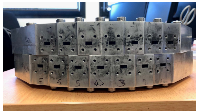
FIGURE 11. Manufactured prototype: (a) View from the array of septum polarizers, (b) View from the input ports.
