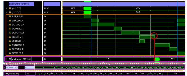
FIGURE 12. Waveforms corresponding to the turbo decoder 1st iteration process.
