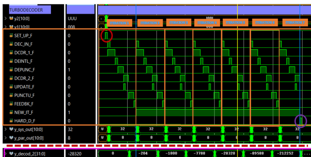
FIGURE 14. Waveforms corresponding to performing the turbo decoder iterations.
