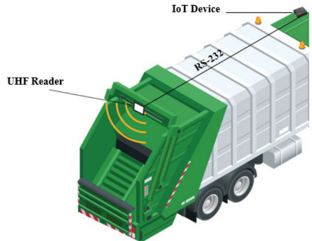
FIGURE 15. Installation of UHF reader and IoT Device.
