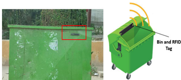
FIGURE 17. Installation of UHF tag over bin.
