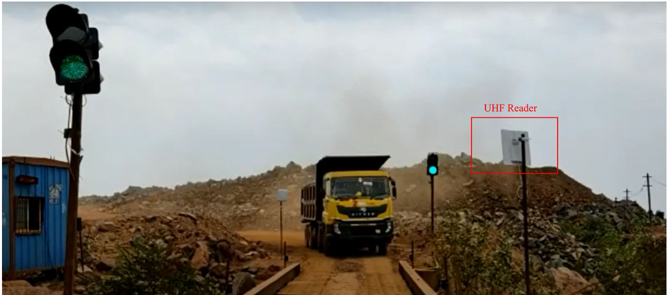
FIGURE 24. Real-time image of dumping waste and UHF detection.
