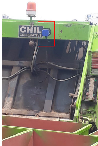
FIGURE 16. Real-time installed UHF reader.
