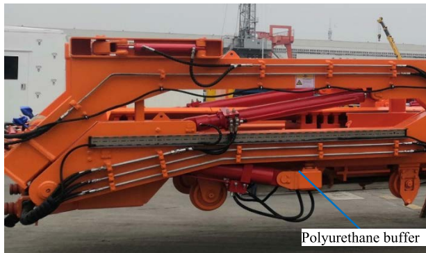
FIGURE 16. A buffer design added to the retracted limit position of the centralizer arm.
