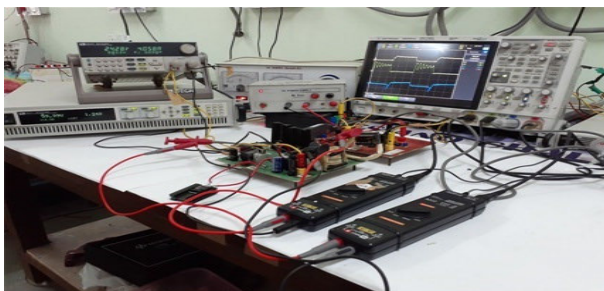
FIGURE 18. Experimental set up of proposed soft switched buck converter.
