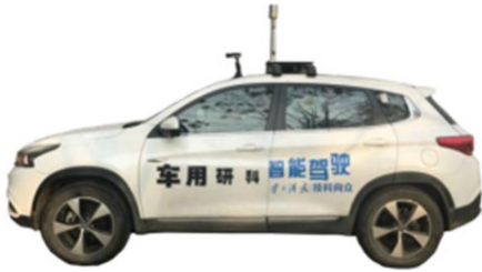
FIGURE 5. Self-driving car 'Tu Lian' with the camera mounted in the vehicle for data collection. POINT GREY BFLY-PGE-23S6C-C camera sensor was mounted in the 'Tu Lian' for data collection.
