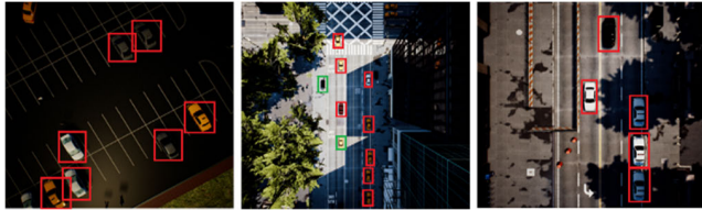
FIGURE 5. Vehicle detection over a few images of the DLR3K complex aerial images dataset.
