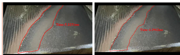
FIGURE 13. Image recognition system (the first image is the previous feature recognition effect of mineral ore belt image, and the second is the under the tabling operation parameters have been optimally tuned).
