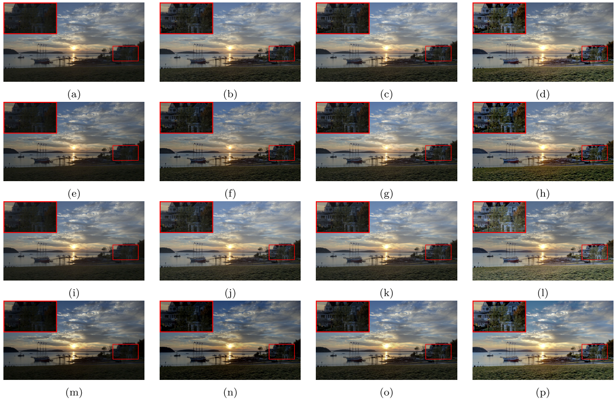
FIGURE 13. Comparison of three segmentation methods (Approach A, Approach B, and proposed scene segmentation method) for Bar Harbor Sunrise. (a)-(d) are the results with Mertens et al.'s fusion method [9] for w/o SSLA, A (CE), B (CE), and Pr. (CE), respectively. (e)-(h) are the results with Nejadi et al.'s method [12] for w/o SSLA, A (CE), B (CE), and Pr. (CE), respectively. (i)-(l) are the results with Kou et al.'s method [13] for w/o SSLA, A (CE), B (CE), and Pr. (CE), respectively. (m)-(p) are the results with Li et al.'s method [17] for w/o SSLA, A (CE), B (CE), and Pr. (CE), respectively.
