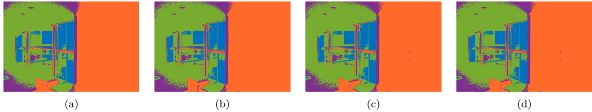
FIGURE 7. Scene segmentation results of the proposed method for the multi-exposure image shown in Fig. 1. (a) Without CE, (b) with CE (bilateral filter), (c) with CE (guided image filter), (d) with CE (weighted guided image filter).
