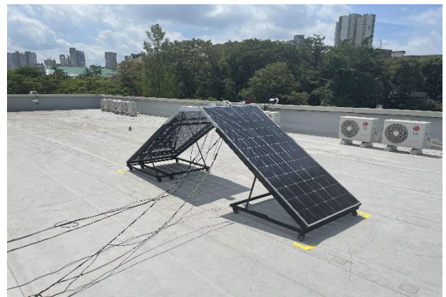
FIGURE 8. PV power system with 0.66 kW Bi-EW.
