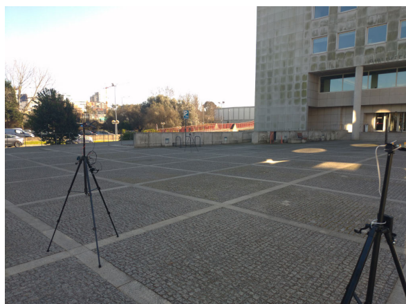
FIGURE 25. Photographs of experimental setup for data collection of 600 packets per each 21 test locations of the 12 by 12 meter test area.
