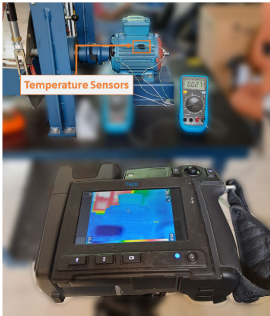
FIGURE 6. Temperature sensors and FLIR thermographic camera setup.
