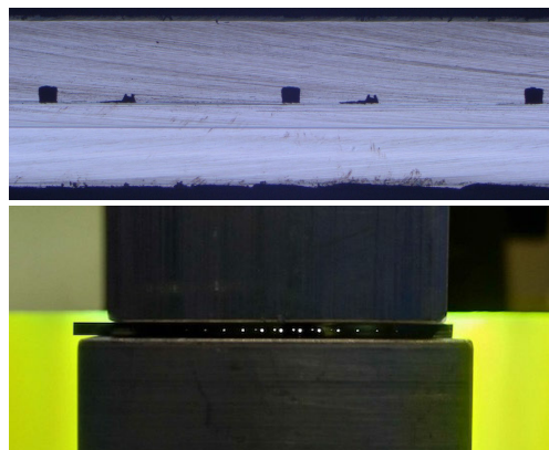
FIGURE 9. SEM based cross-section of semiconductor tubes (top) with 100 \times 100\mu\text{m}^2 and 30 \times 30\mu\text{m}^2 core regions stacked adjacent to each other in a 3mm end-to-end zoomed-in field-of-view. Light passing through the length of these tubes (bottom).
