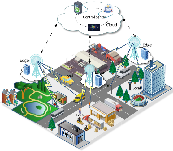
FIGURE 1. Illustration of the SAHFL based mobile edge networks.
