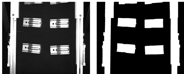
FIGURE 3. Binary preprocessing of the image to be tested.
