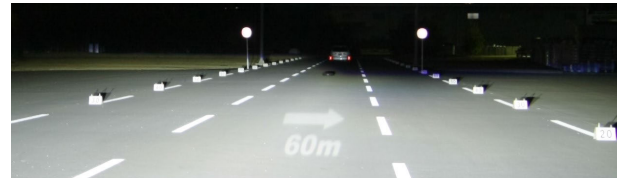
FIGURE 1. Examples of a road projection lamp. The road projection lamp indicates navigation information.
