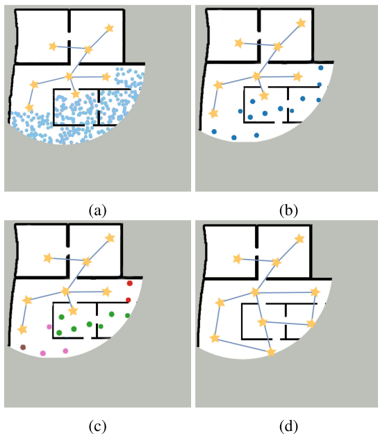
FIGURE 3. The process of incremental segmentation during exploration: (a) Points sampling in the partially known area; (b) Lower level clustering and (c) Lower and Upper level clustering on the partially known area; and (d) Incremental graph construction based on the growing segment clusters.
