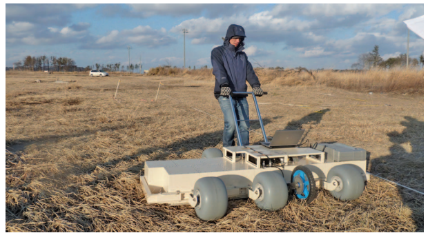
FIGURE 6. GPR system "Yakumo" newly developed to accelerate archeological survey required for re-establishing towns on offshore uplands. Courtesy of Tohoku University.
