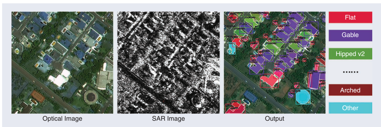
FIGURE 2. An example image tile of the provided multimodal data (optical and SAR) for building detection and roof type classification.
