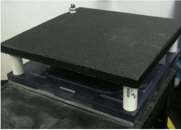
Fig. 10. WPT coupler (specifications in Table II) used for simulation and its characterized coupling coefficient, k_z [5].
