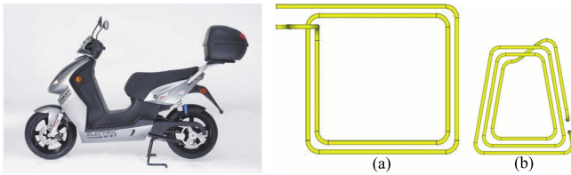
Fig. 23. Windings used in the wireless charger for E-scooters [79], [84] (Copyright @ IEEE). (a) Transmitter coil. (b) Receiver coil.
