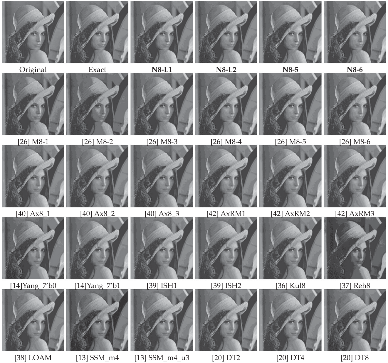
FIGURE 11. Gaussian smoothing of images obtained with different multipliers. The circuits proposed in this paper are highlighted in bold.
