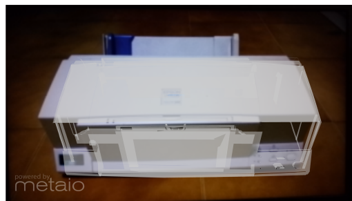
FIGURE 2. A representation of the 3D model helps the user to correctly align the device's camera with the real object.
