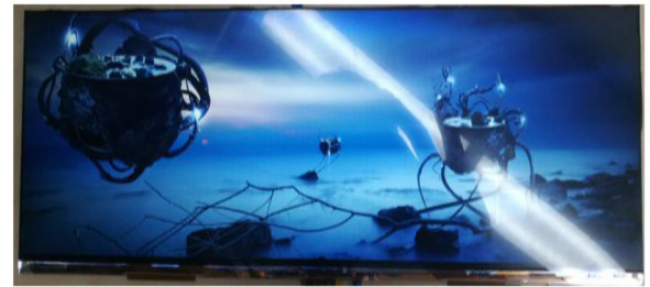
FIGURE 9. Photo image of the fabricated 12.4-inch nearly-bezel-free LCD panel based on the GIA integration.
