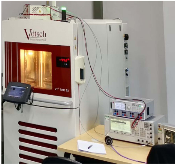
FIGURE 3. Thermal shock test environment.
