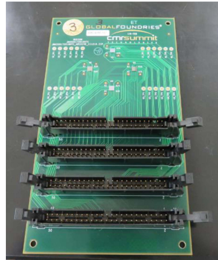
FIGURE 5. TCoB test board with 4 dies and 4 connectors mounted.
