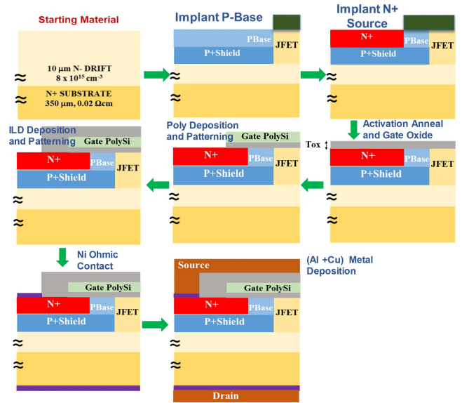
FIGURE 2. PRESiCe™ technology process sequence for manufacturing the SiC power MOSFETs.
