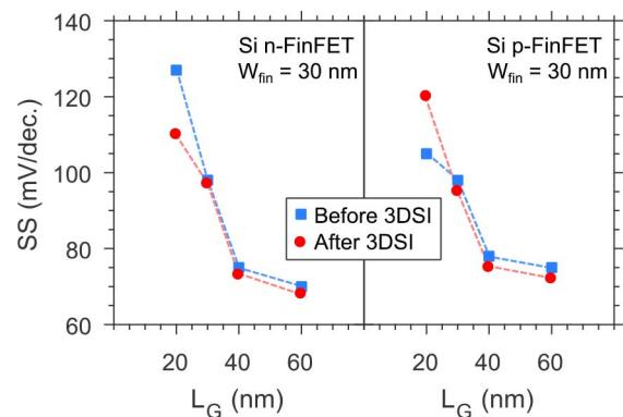
**FIGURE 5.** Subthreshold slope of Si CMOS n- and p-FinFETs in saturation, for devices with fin width of 30 nm before and after 3D sequential integration of the top III-V transistor layer. Negligible change of SS is observed as a result of the 3DS integration.
