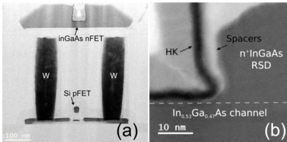
**FIGURE 2.** a) STEM cross-section of the 3DS integrated stack showing both transistor levels. Cross-section along the gate showing an InGaAs nFET with  $L_G = 60$  nm on top of a Si pFET. W inter-layer contacts are also shown. b) Detailed STEM image of the InGaAs FET gate region featuring design A. High crystalline quality for the InGaAs channel is shown. The Al<sub>2</sub>O<sub>3</sub>/HfO<sub>2</sub> gate oxide and the approximately 4 nm thick SiN<sub>x</sub> spacers are highlighted.
