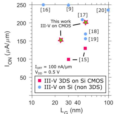
**FIGURE 10.** Benchmarking of  $I_{ON}$  versus  $L_G$  for 3DS integrated III-V FETs on Si (purple symbols) as well as non-3DS III-V on silicon (blue dots) works.
