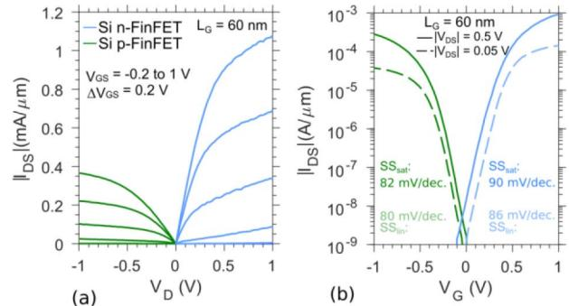
**FIGURE 4.** a) Output characteristic and b) subthreshold characteristic of Si n-FinFET (blue) and p-FinFET (green) with  $L_G = 60$  nm after top-layer 3DS integration.
