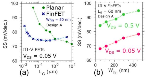
**FIGURE 8.** For design A, a)  $SS_{LIN}$  versus  $L_G$  for planar (green) and FinFETs (blue) structures. b)  $SS$  in linear and saturation region versus fin width.
