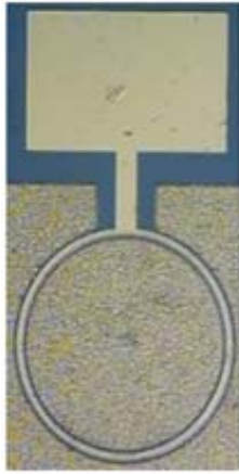
FIGURE 1. Circular FET test structure of 85/70 HEMT.
