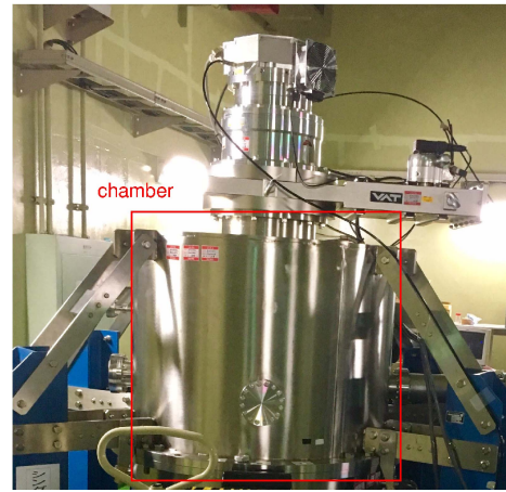
FIGURE 7. Heavy-ion irradiation setup.
