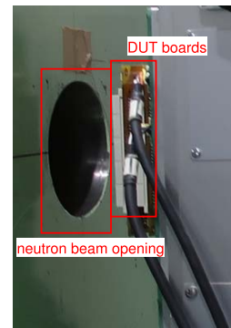
FIGURE 8. Spallation neutron irradiation setup.
