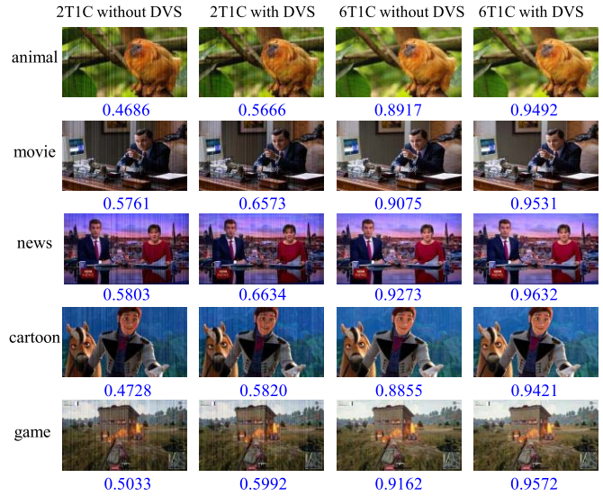
FIGURE 7. Comparison of the reconstructed images using the DVS approach with different pixel circuit designs for various input images. The structural similarity index (SSIM) values were obtained to quantitatively measure the similarity between the reconstructed images and the original ones.
