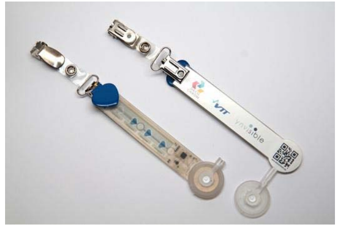
FIGURE 5. Finalized personal activity meters.
