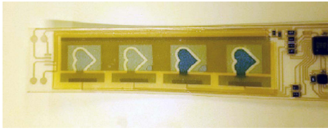
FIGURE 9. Coloring of the spacer foil during the environmental stability test.
