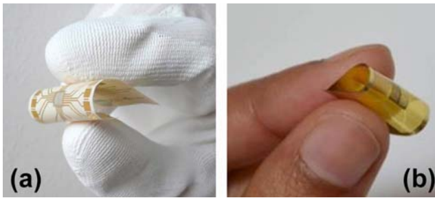
FIGURE 6. Examples of chips ( 4.6 \times 4.6 \text{ mm}^2 , 20 \text{ }\mu\text{m} thick) directly embedded into (a) a flexible LCP [18] ( 20 \times 20 \text{ mm}^2 , thickness 70 \text{ }\mu\text{m} ) or (b) by using CFP interposer technology ( 15 \times 15 \text{ mm}^2 , thickness 60 \text{ }\mu\text{m} ).
