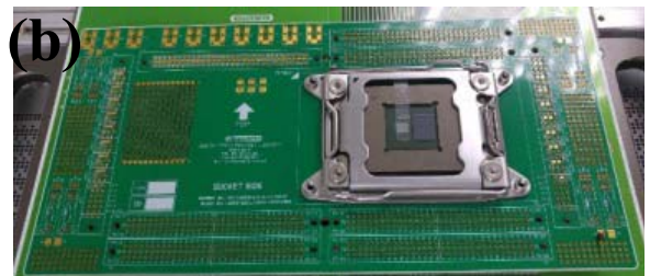
FIGURE 9. 3D stacked DRAM (a) on substrate, and (b) on board for signal measurements.
