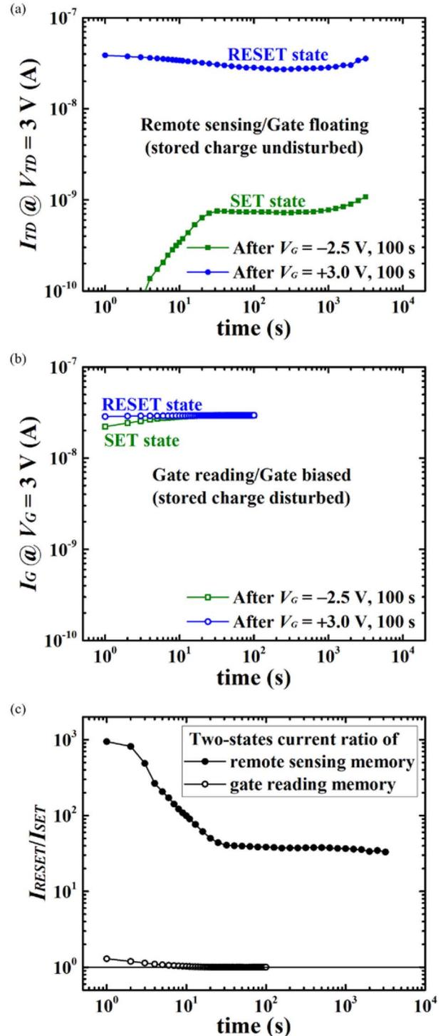
**FIGURE 7.** The measured retention of the set and reset current states read at (a)  $V_{TD} = 3$  V and (b)  $V_G = 3$  V. (c) The extracted current ratios of set and reset states in (a) and (b).
