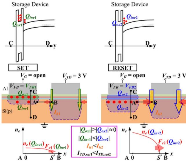
**FIGURE 8.** The schematic diagrams of the read mechanism in Fig. 9(a). Left: the read process after the gate was set ( $V_G = -2.5$  V, 100 s). Right: the read process after the gate was reset ( $V_G = +3.0$  V, 100 s).  $x = S^*$  is the position at the depletion edge of the MIS TD.
