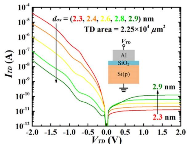
**FIGURE 1.** The measured current-voltage characteristics of p-type MIS TD's with various oxide thicknesses. The inset shows the MIS TD structure (Al/SiO<sub>2</sub>/Si(p)).
