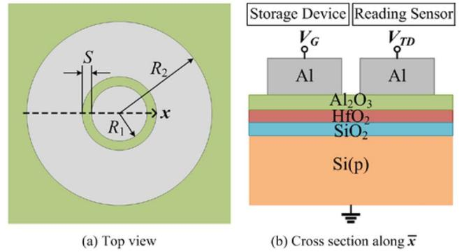
**FIGURE 5.** Schematic (a) top view and (b) cross section of the gated-MIS TD.
