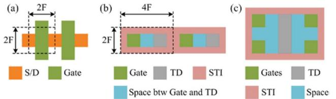
**FIGURE 10.** (a) The layout of conventional NAND flash memory cells. (b) The compact layout of proposed memory cells. (c) The layout of the proposed memory cell with multi-gate structure (four gates are illustrated as an example).
