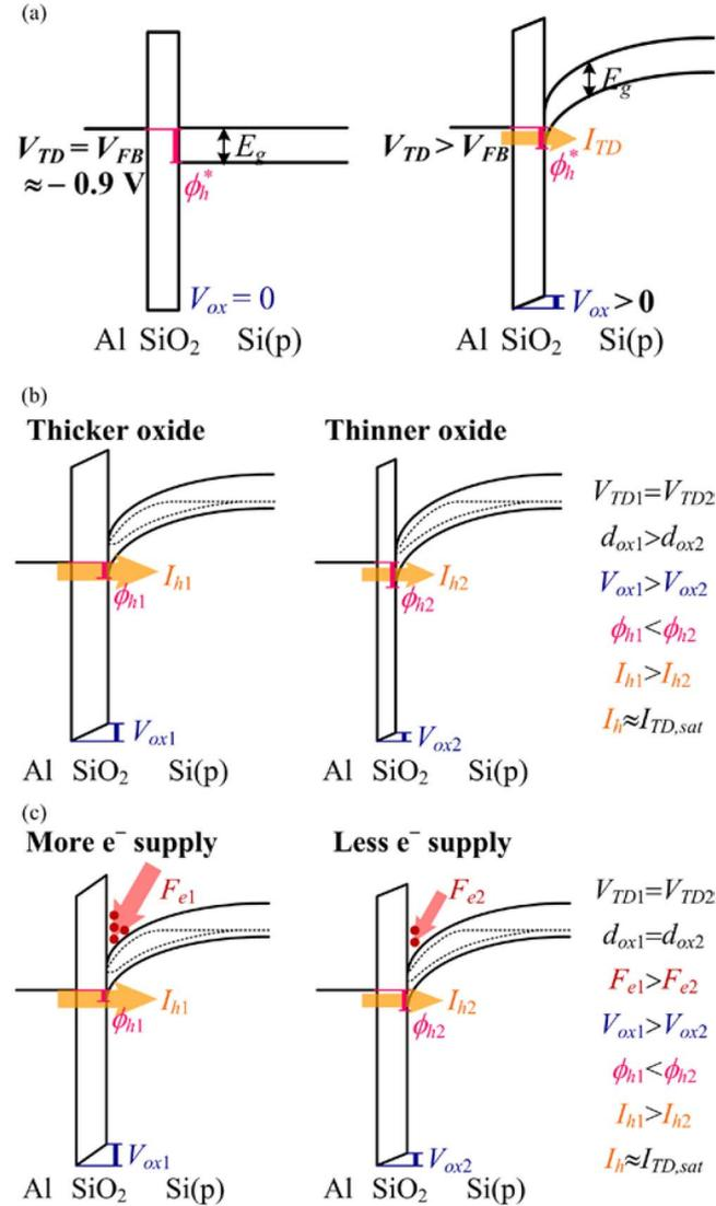
**FIGURE 2.** (a) The band diagrams of p-type MIS TD's at flat-band ( $V_{TD} = V_{FB}$ ) (left) and  $V_{TD} > V_{FB}$  (right). (b) The band diagrams of p-type MIS TD's with thicker oxide (left) and thinner oxide (right).  $I_h$  is the hole current.  $I_{TD,sat} \approx I_h$ . (c) The band diagrams of p-type MIS TD's while the lateral electron flux is large (left) and small (right).
