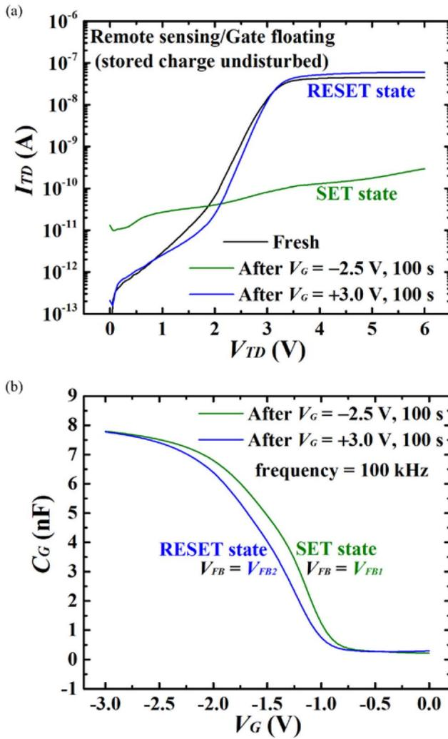
**FIGURE 6.** (a) The measured current-voltage characteristics of the MIS TD as the gate is at fresh, after the write voltage stress ( $V_G = -2.5$  V, 100 s), and after the erase voltage stress ( $V_G = +3.0$  V, 100 s). (b) The measured gate capacitance,  $C_G$ -voltage curves at 100 kHz after the write and erase processes.
