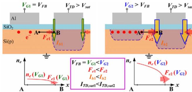
**FIGURE 4.** The schematic operations of gated-MIS TD as the gate was biased at flat-band ( $V_G = V_{FB}$ ) (left) and  $V_G > V_{FB}$ .  $n_e$  is the minority carrier concentration along the cross section AB.
