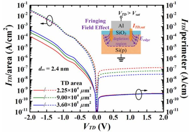
**FIGURE 3.** The measured current-voltage characteristics of MIS TD's with various device areas. The dotted lines are the currents per unit device area, and the solid lines are the currents per unit device perimeter. The inset shows that the saturation current of MIS TD is mainly flowing through the edge of the device due to the fringing field effect.  $E_{edge}$  is the fringing electric field.
