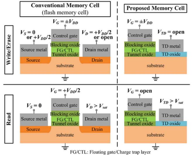
**FIGURE 9.** The schematic diagrams that compares the applied voltages of write/erase and read operations of the conventional flash memory cell with that of the memory cell with MIS TD sensor proposed in this work.
